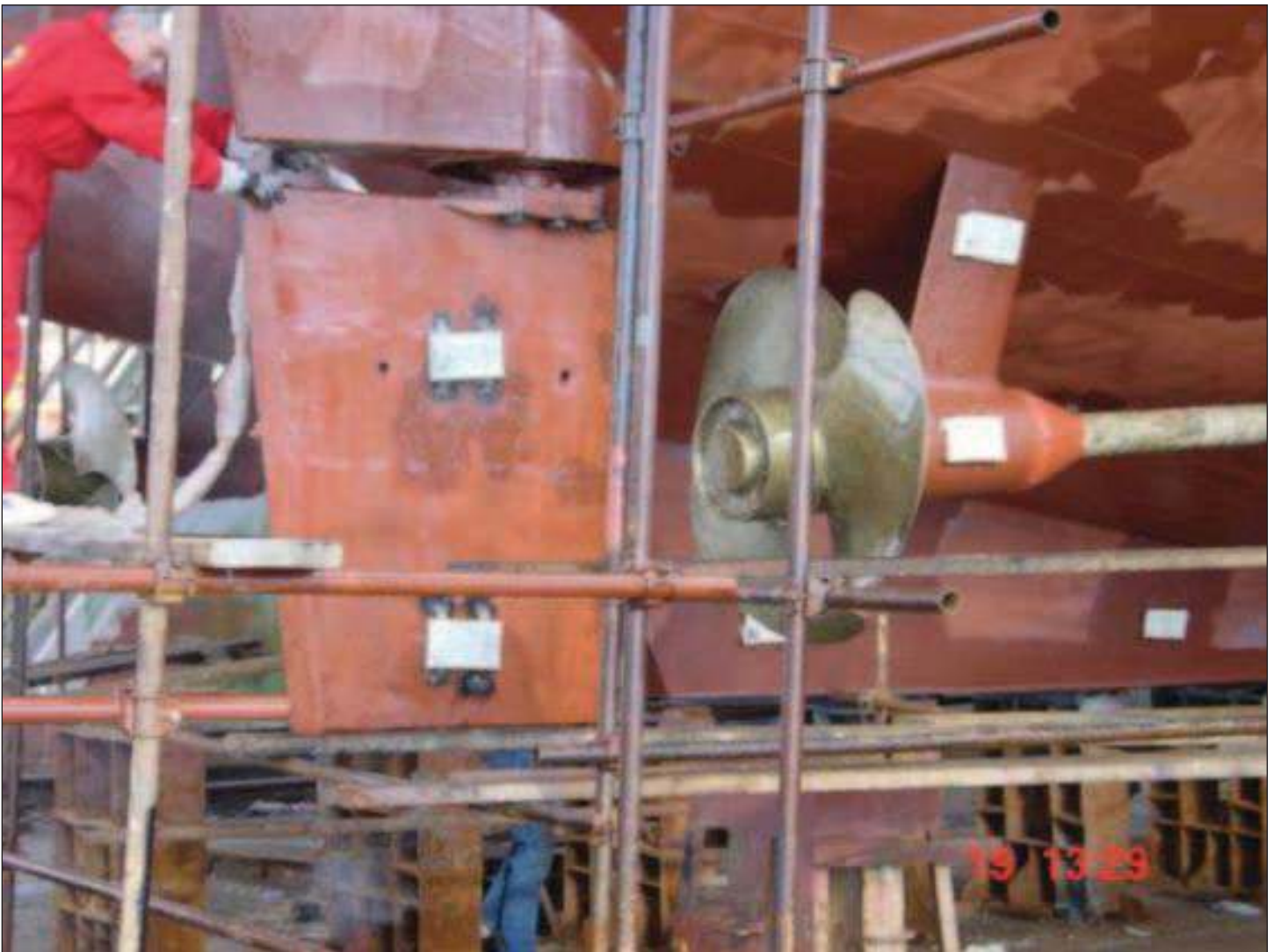
Figure 3. Protection of the rudder blade with VpCI®
