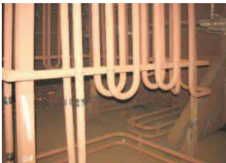
Figure 9. SHIP - ASPHALT CARRIER, 12 asphalt storage tanks /1 tank = 1000 m 3 , VpCI 645 (100 ml/m 3 per tank)
