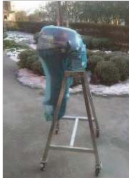
Figure 16. Outboard engine wrapped in VpCl® Film
