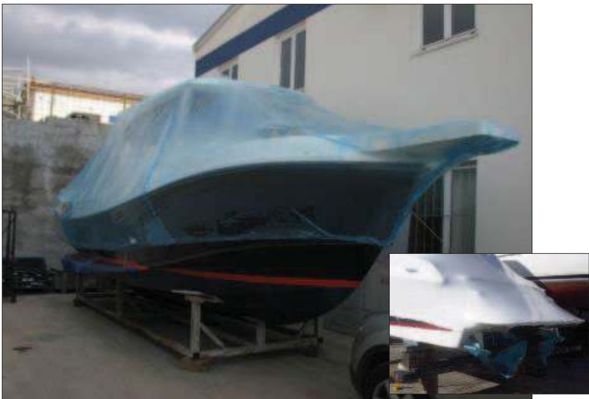
Figure 17. Corrosion protection of yacht on dry berth located on coastal area of Croatia
