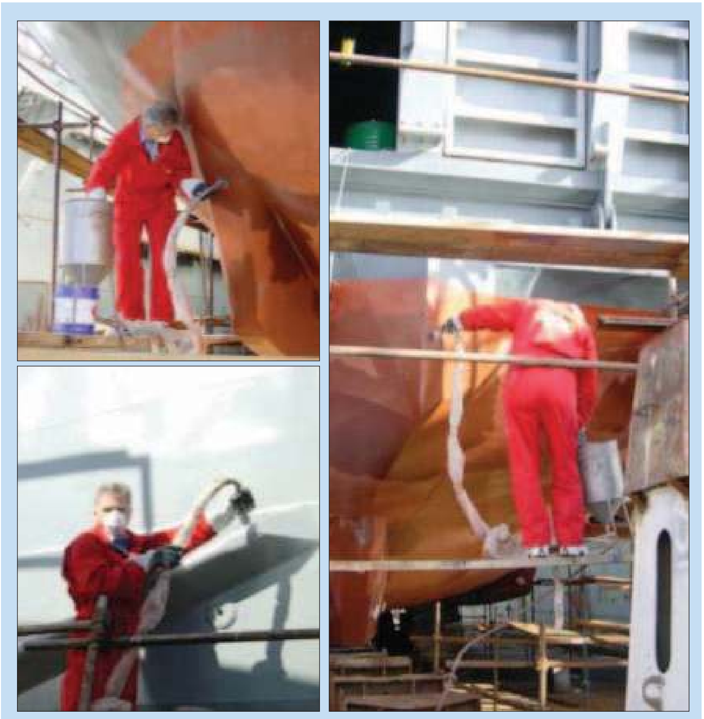
Figure 6. Application of VpCI® inhibitor to keel, rubbing strip and bow of the boat.
