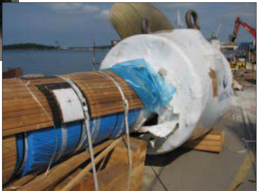
Figure 8.b Protection of equipment with VpCl® 126 film
