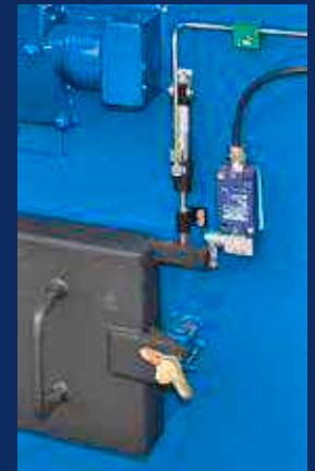
Safety devices prevent unintentional opening of doors
